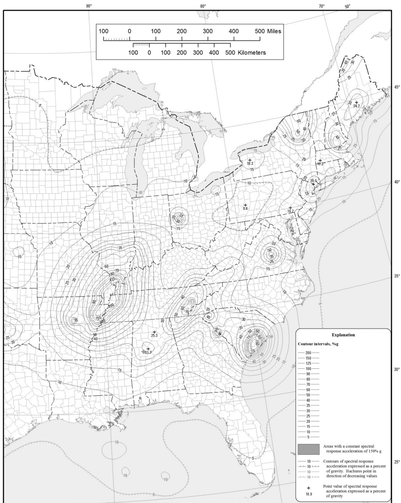
FIGURE 1613.2.1(1)—continued RISK-TARGETED MAXIMUM CONSIDERED EARTHQUAKE (MCE R ) GROUND MOTION RESPONSE ACCELERATIONS FOR THE CONTERMINOUS UNITED STATES OF 0.2-SECOND SPECTRAL RESPONSE ACCELERATION (5% OF CRITICAL DAMPING)
