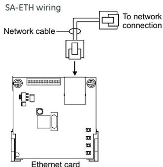
The SA-ETH card provides a standard 10/100 Base T Ethernet network connection for connecting to an intranet, a local network, or the Internet. The card can be used to download configuration programming from the VS-CU to the panel over the network.
