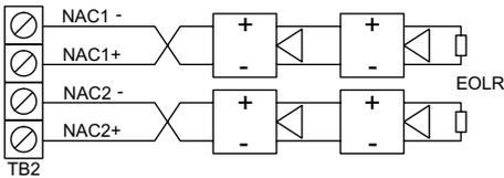
Marking indicates output signal polarity when the circuit is active. Polarity reverses when the circuit is not active. Wire notification appliances accordingly. Notification appliance polarity shown in active state.
