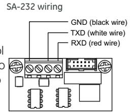
The RS-232 card is installed on the plastic assembly and connects to the main circuit board via a ribbon cable.
