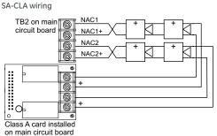
even though this wiring does not return to the SA-CLA card. The SA-CLA is compatible with VS1 control panels only. VS2 panels are Class A ready. The SA-CLA is installed directly to the control panel circuit board using its plastic standoffs and plug connection.
