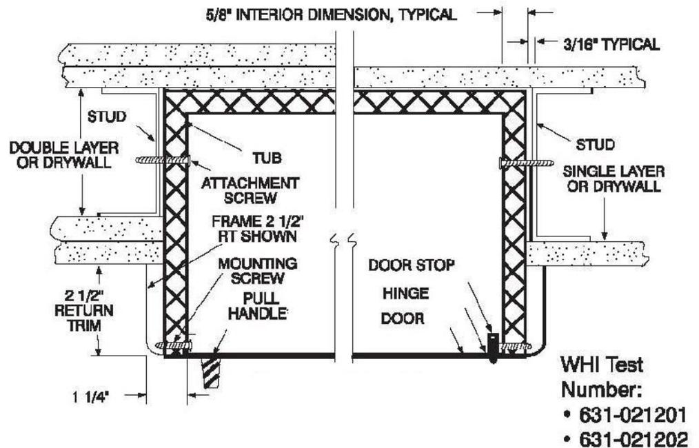
**NOTE:** The installation of any fire-rated cabinet which lacks a cabinet door, or any condition in which the door is left ajar, will void the fire rating
